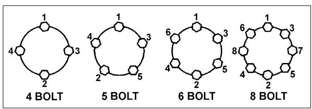
Lug Nut Sequence of Tightening - Figure 8-8
