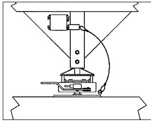
Breakaway Brake Connection - Figure 3-22
