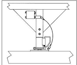
Breakaway Brake Connection - Figure 3-16
