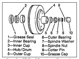
Standard Wheel Bearing - figure 8-5 Follow the steps below to disassemble and service the wheel bearings.
