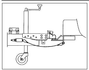
Breakaway Brake Connection - figure 3-8
