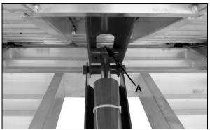
Lube Hydraulic Cylinder Pin - Figure 8-3
